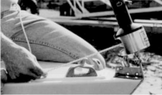
Locating the first fairlead
