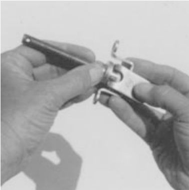
T-bolt/toggle with spacer washers and antirotation strap in place
