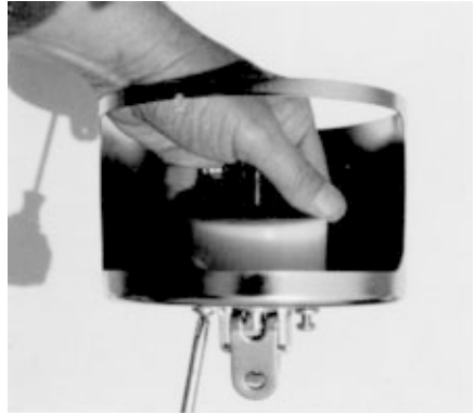
Assembling cup, bearing and antirotation strap
